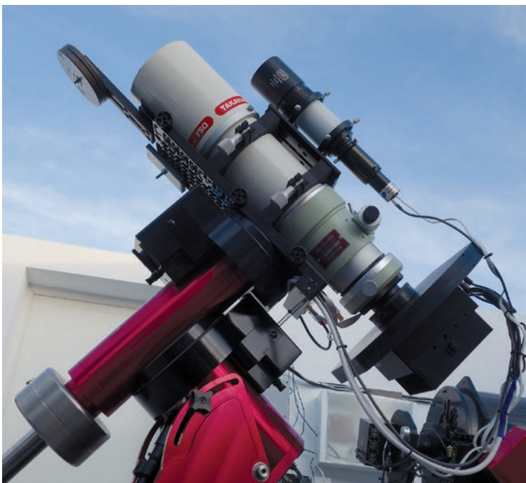
■ Fig 5. Also located at IC Astronomy in Spain are two Takahashi FSQ-106 premium refractors on Paramount MX+ mounts (SPA-1 and SPA-3). The image of the North America Nebula in Cygnus was taken using SPA-1 and consists of just 2 \times 10 minute exposures per narrowband filter.
