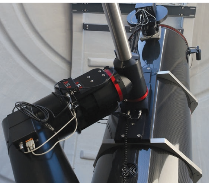
■ Fig 3. Telescopes CHI-2 and CHI-4 are two superb 500mm corrected-Newtonian reflectors with fast f/3.8 optics suitable for highly detailed wide-field imaging. On the right is a view of the Tarantula Nebula in the Large Magellanic Cloud, in the southern constellation of Dorado, as captured by the CHI-2/4 instrumentation. Exposures were: luminance, 3 × 10 minutes; RGB, 2 × 10-minutes per filter.
