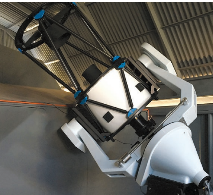
■ Fig 2. CHI-1 is a 600mm Planewave Corrected Dall–Kirkham telescope. The image on the right is of the enigmatic nebula NGC 3576 in the southern constellation of Carina, taken with the CHI-1 instrumentation. The narrowband image was achieved using 3nm Astrodon filters. Exposures were: hydrogen-alpha, 3 × 10 minutes; oxygen-III, 4 × 10 minutes; and sulphur-II, 4 × 10-minutes.
